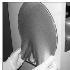
Tighten fabric while making it slip downward.
