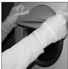
Put the fabric around the ring, starting from top. Make sure that the rubber band goes between the aluminium profile and the cabinet.
